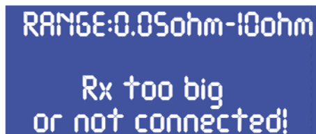
Fig.14 Mode CR injector R meter – Rx exceeds the measurement range
