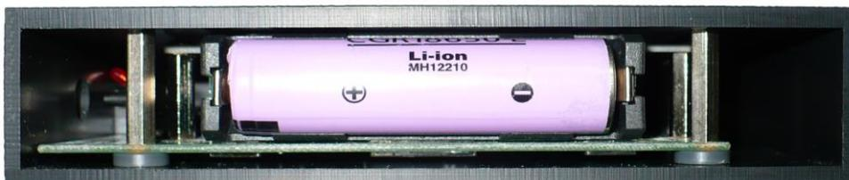
Note: After installing or replacing the battery you should set actual date/time by going to: Home screen>Settings>Date & Time
