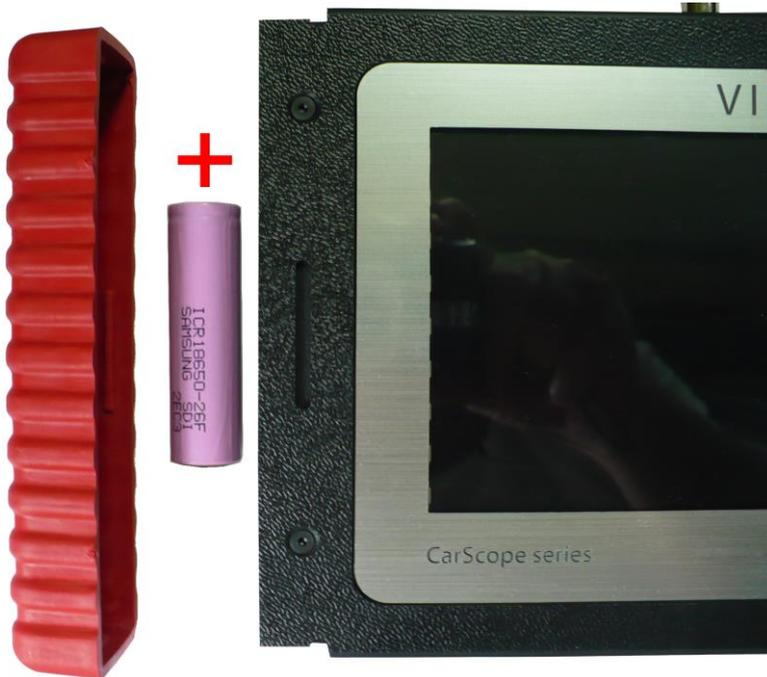
CarScope VISO uses a rechargeable Li-ion battery 18650 type, 2600mAh capacity. To install the battery do the following:
