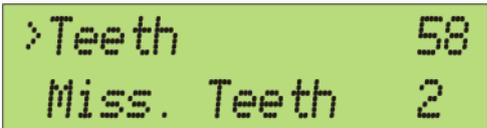
Fig.11 CKP Setup Menu – Adjust the number of teeth
