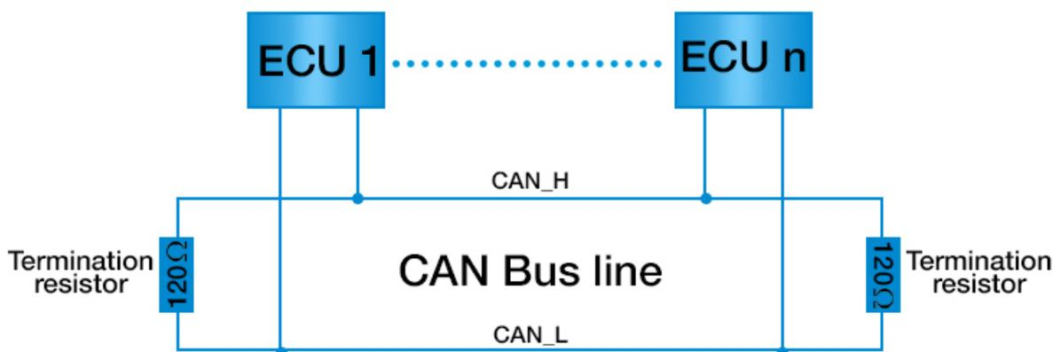
For low-speed CAN, the impedance is close to 100 Ohm but not less than that.
