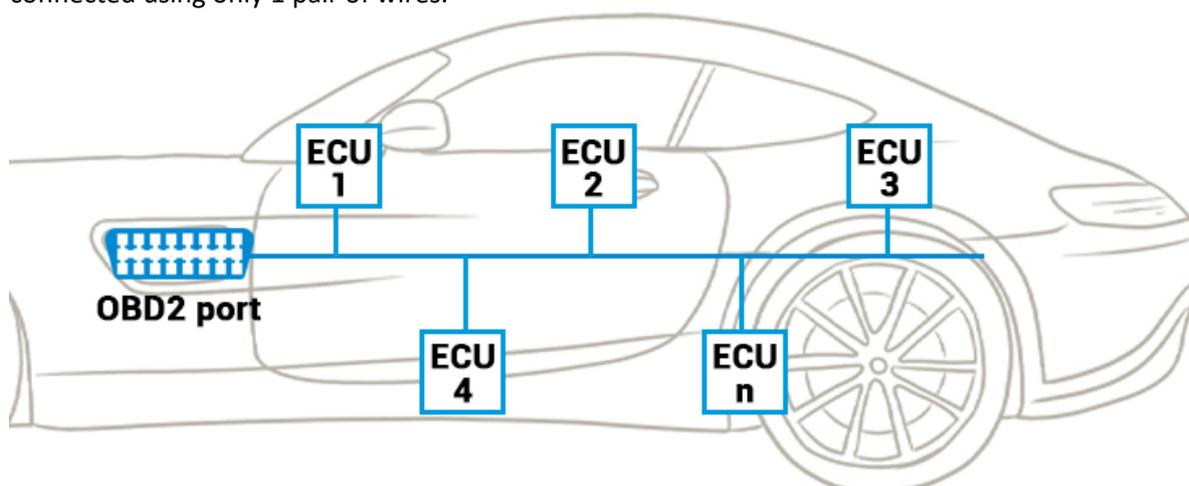
Modern cars nowadays can have up to 80 ECUs, just imagine how messy and costly it is to connect these modules to each other using analog signal lines.
