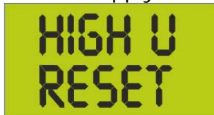
Fig.7 High voltage protection is activated – power supply voltage is more than 16V
