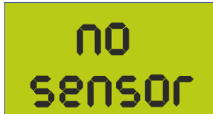
Fig.8 Pressure sensor failure or pressure sensor is not connected. This protection activates if sensor output is less than 0.35V when pressure is 0bar.
