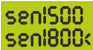
Fig.1 Main menu – default mode is CP3 Pump & Rail Pressure Valve and default sensor is 1800bar (sen1800) .
