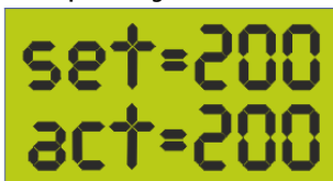
Fig.2 CP1 Pump Control Valve mode – Set pressure is 200bar and actual pressure is 200bar.
