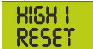
Fig.5 Overcurrent or output short circuit protection is activated
