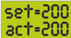
Fig.3 CP3 Pump & Rail Pressure Valve mode – Set pressure is 200bar and actual pressure is 200bar.
