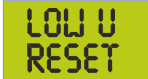
Fig.6 Low voltage protection is activated – power supply voltage is less than 11V
