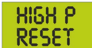
Fig.4 Overpressure protection is activated – rail pressure has exceeded 1470bar for a 1500bar pressure sensor or 1750bar – for 1800bar pressure sensor
